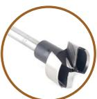
**1 1/4" Forstner or Spade bit – ONLY REQUIRED for hard wood posts OR if you encounter a problem of post splitting.** A Forstner bit cuts easier than a spade bit and is used to remove some of the wood so the hole saw can be used for a second deeper pass. **Please see Special Instructions.**
